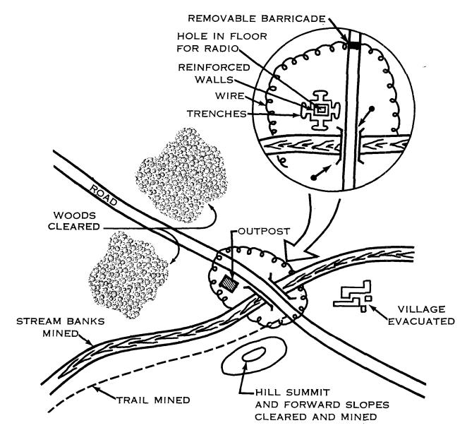
Figure 9. Typical static security post (guarding bridge).
