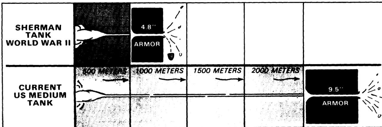
The Sherman tanks of General Patton's Third Army had to close to within 500 meters of the German PzV Panther tank before the American 76mm gun could punch through the German's 4.8 inches of frontal armor. Current US medium tanks can penetrate nearly twice that much armor at four times the range.
