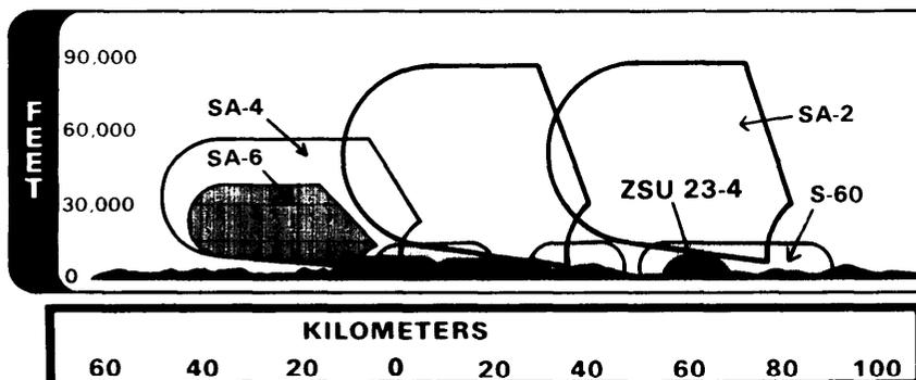
This figure portrays a typical Soviet Combined Arms Army air defense system 50 kilometers wide and 100 kilometers deep. Shoulder-fired SA-7 and vehicle-mounted SA-9 launchers common to all units are not shown, but provide a dense blanket of low altitude air defense which complements the other systems.
