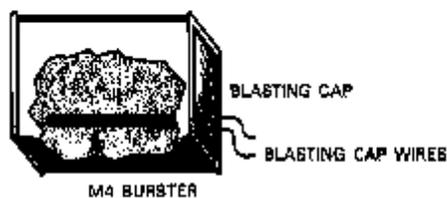
● FRAGMENTATION EXPLODING FLAME DEVICE (EXPLOSIVE CHARGE OR M-4 BURSTER)
