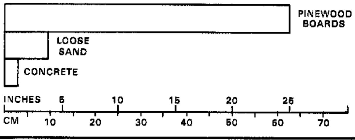
7.62mm ball cartridge penetration at 200m
