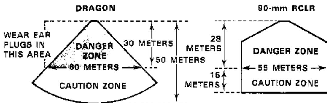
In urban areas, the backblast hazard may be increased by the presence of rubble and the channeling effect caused by narrow streets and alleys. Therefore, friendly troops must be behind protective cover and wear helmets, flack vests, and ear-plugs if they cannot move out of the caution area.
