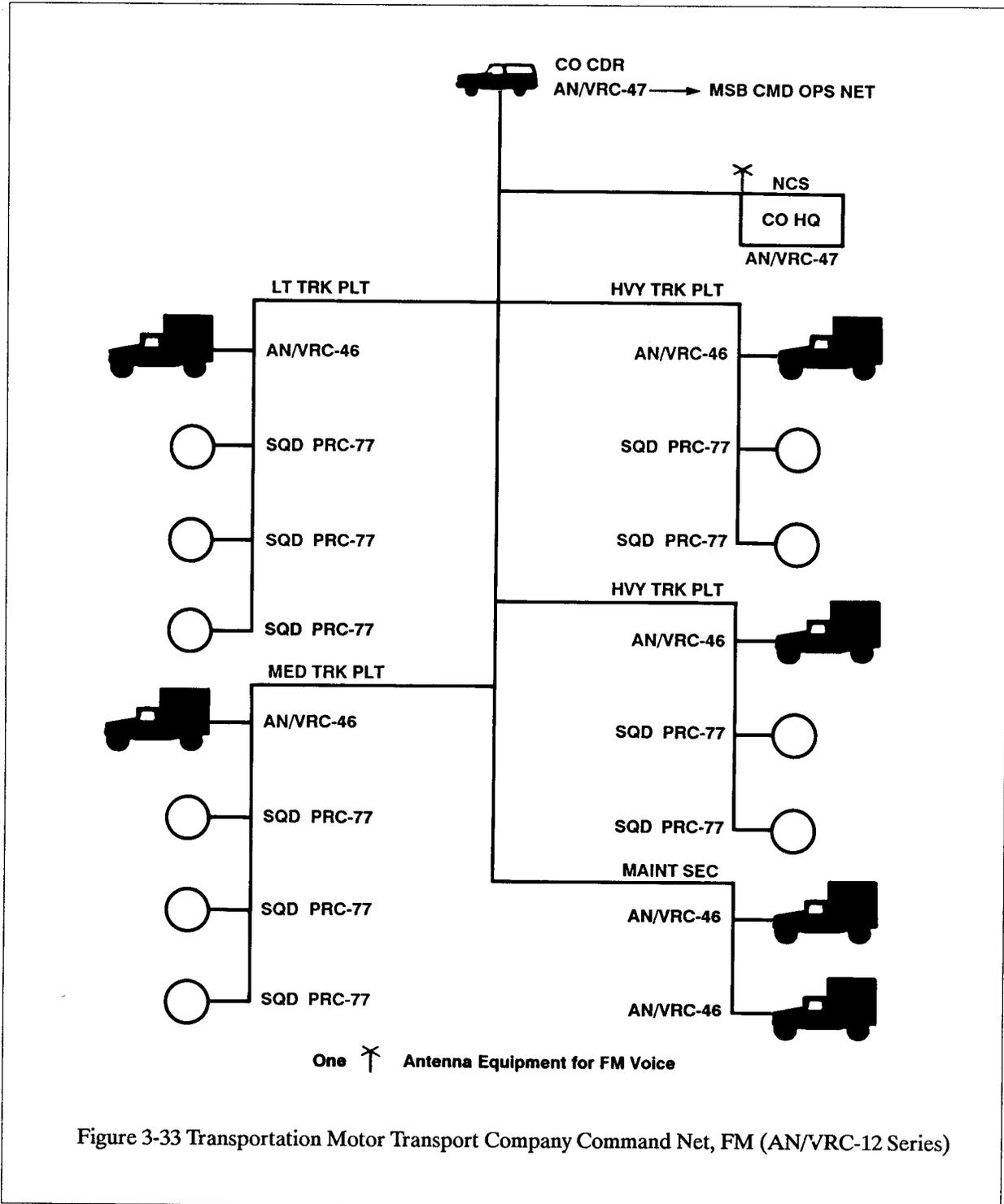
Figure 3-33 Transportation Motor Transport Company Command Net, FM (AN/VRC-12 Series)
