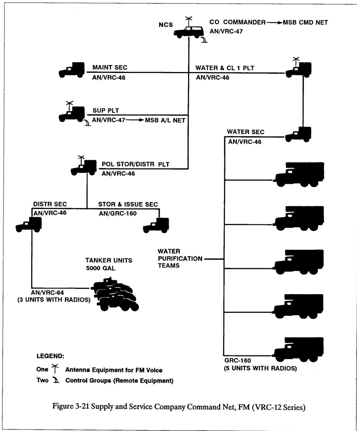
Figure 3-21 Supply and Service Company Command Net, FM (VRC-12 Series)
