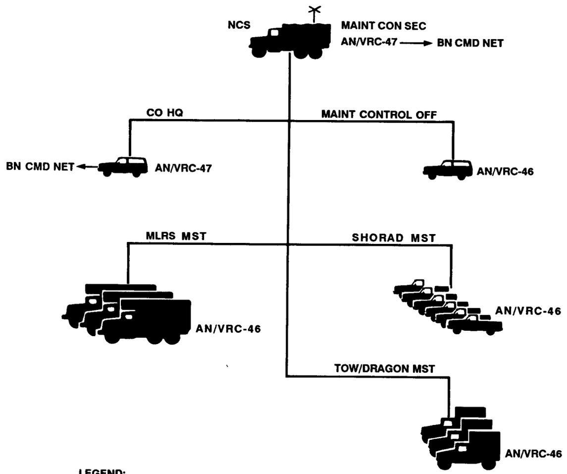
Figure 3-27 Missile Support Company Command Net, (AN/VRC-12 Series)
