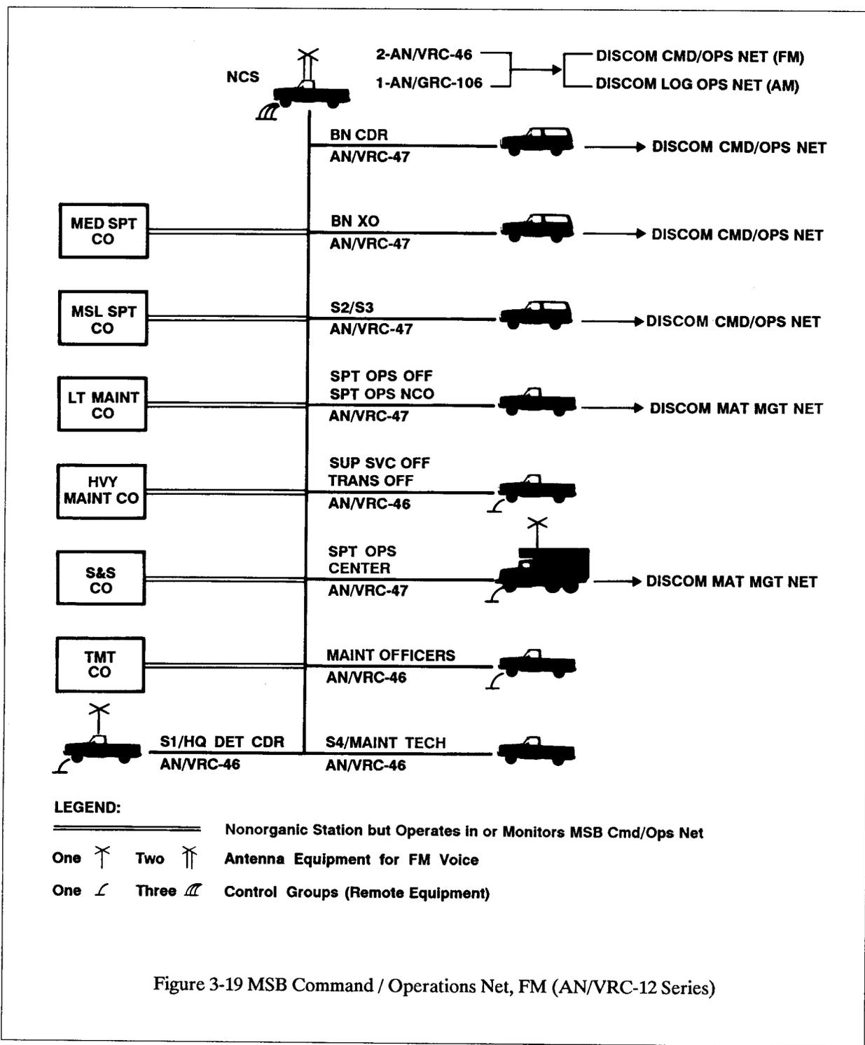
Figure 3-19 MSB Command / Operations Net, FM (AN/VRC-12 Series)
