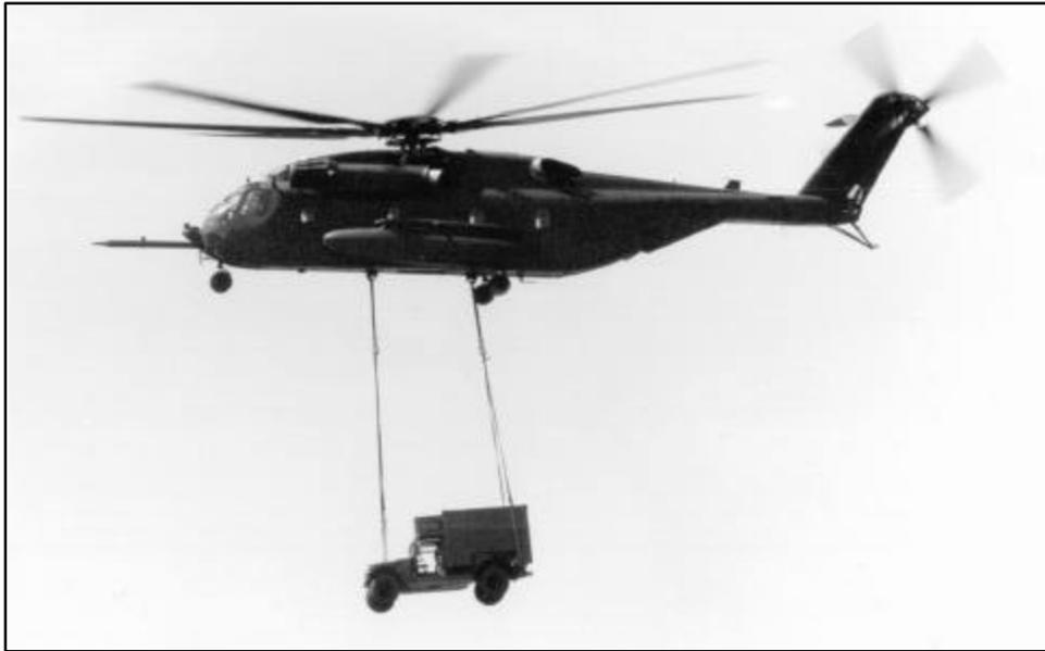
**Figure 2-7. CH-53 Using Cargo Slings**
