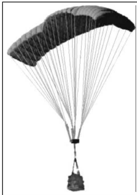
Figure 7-1. Precision Extended Glide Aerial Delivery System (PEGASYS)
