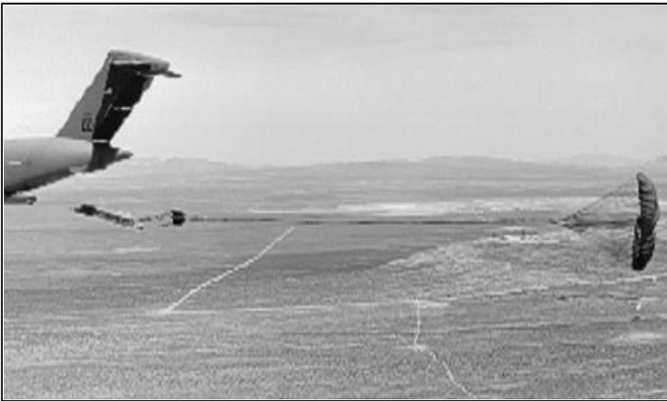
Figure 7-3. The 500-Foot Low Velocity Airdrop System (LVADS)
