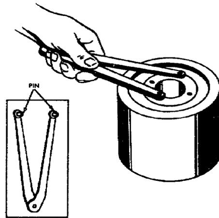
**Figure 19. Using adjustable spanner wrench.**
