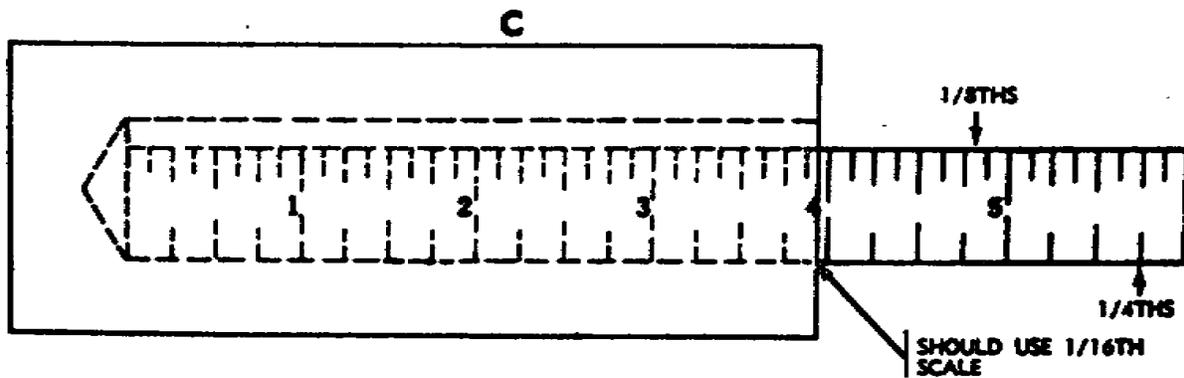
Figure 43. Determining proper graduated rule.
