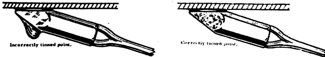
Figure 24. Iron tinned for working on underside:.
