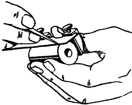
**Figure 48.** Using key seat clamps, rule, and scriber.
