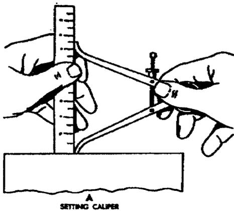
Figure 52. Setting and using inside caliper.
