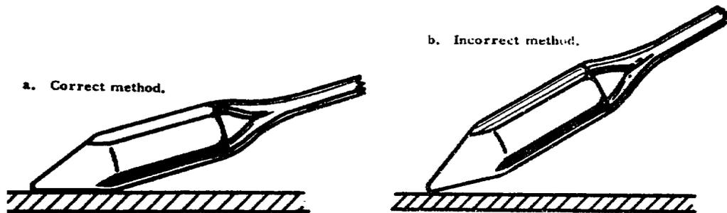
Figure 25. Correct and incorrect methods of using cored solder.
